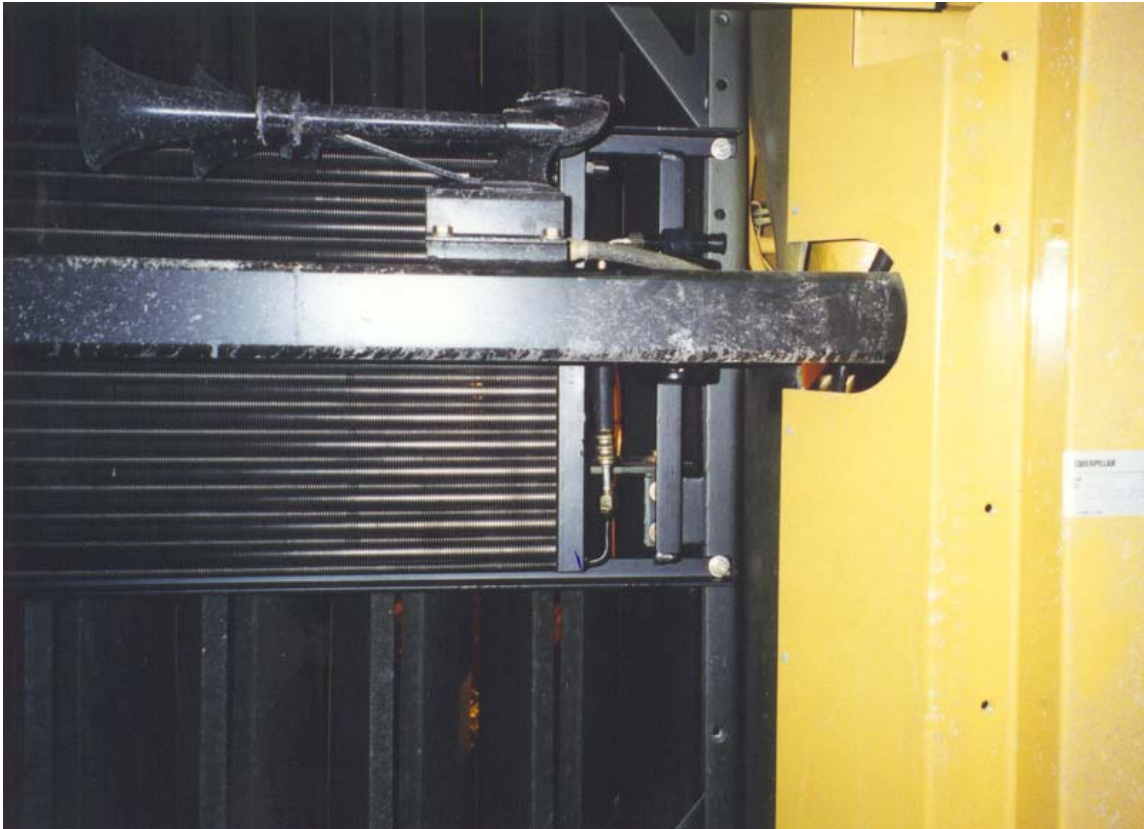
Right side of condenser with drier as viewed from front of truck.
